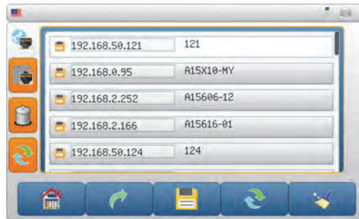
Figure 3.2 Screen showing list of weld controls available on a Global EtherNet Network.
